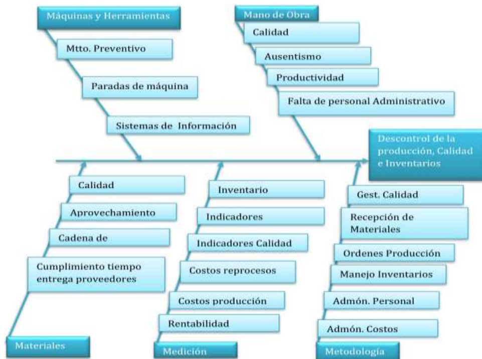
Figure 2: Ishikawa diagram for the fundamental symptom or effect: 'Descontrol of Production, Quality, and Inventories'. (Source: authors)
