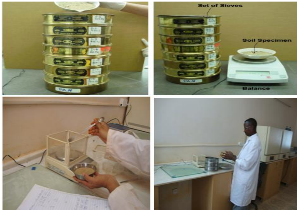
Figure.7 Sieve analysis test procedure
