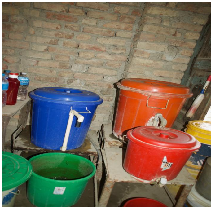
Figure 1. KAF with the outlet lower than the nail bed (red filter, old system) as well as the modified version of aKAF with the higher outlet (blue filter). Photo: B. Mueller, 9.4.2021.
