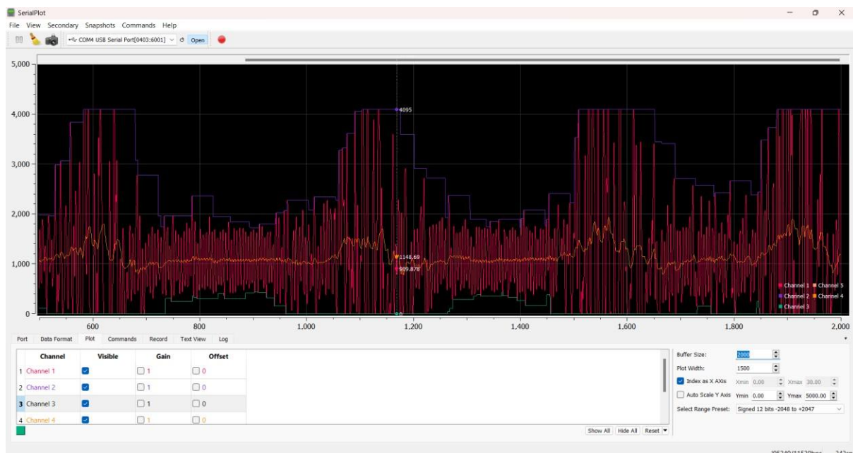
Figure 36: USB-UART Output data live streaming from EMG Click – MCU [12]
