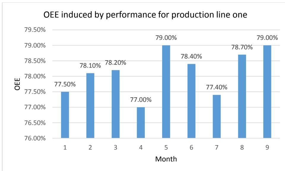
Figure (3.3) Monthly OEE induced by performance for production line one along nine months
