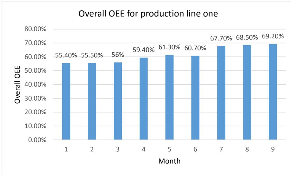
Fig (3.7) Monthly overall OEE for production line one along nine months
