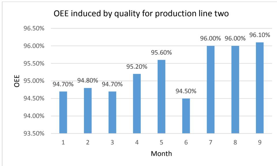
Fig (3.6) Monthly OEE induced by quality for production line two along nine months.
