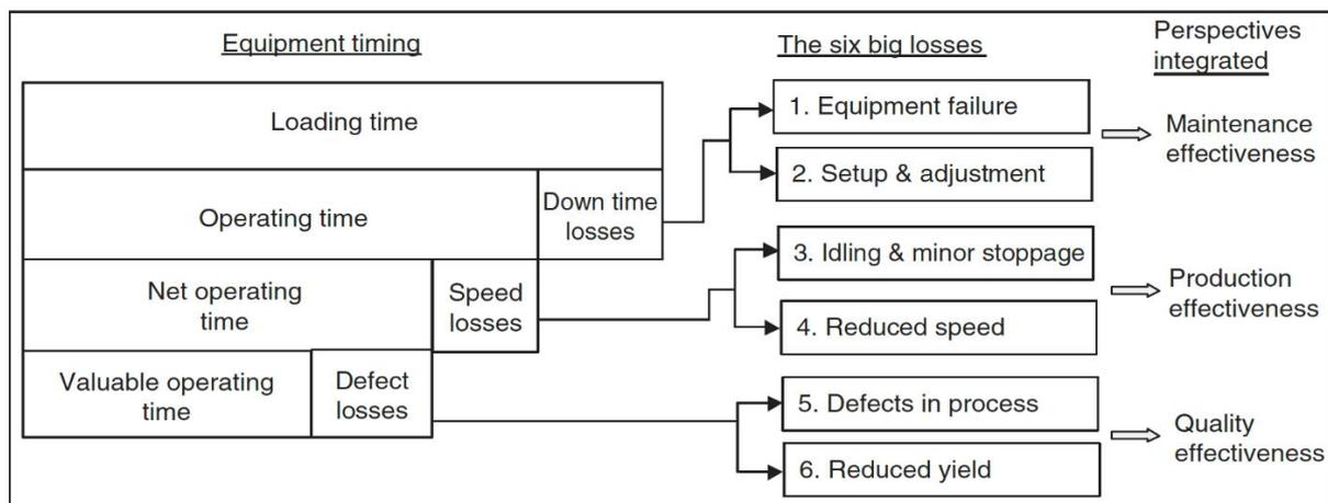
Figure (1.1) OEE measurement tool and the perspectives of performance integrated into the tool [10].
