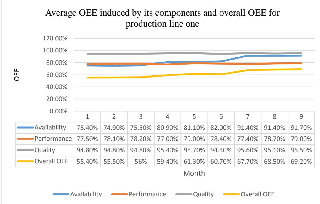
Figure (3.9) Variation in average OEE and corresponding overall OEE along nine months for production line one
