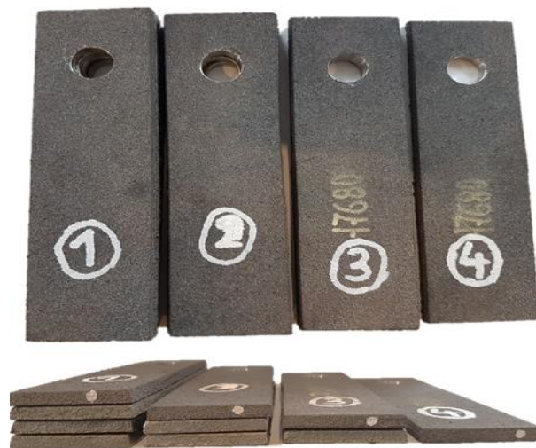
Figure 7: Cast disintegration hammers from different material compositions [8]
