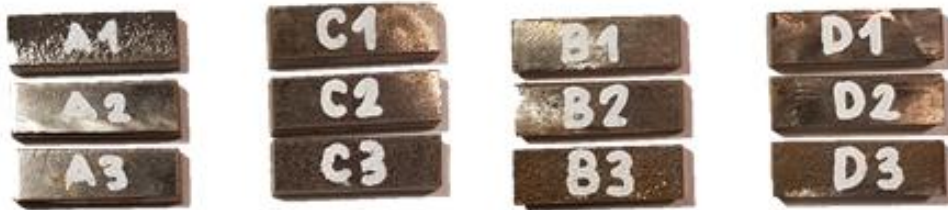
Figure 11: Prepared testing specimens for measuring of adhesive wear [8]
