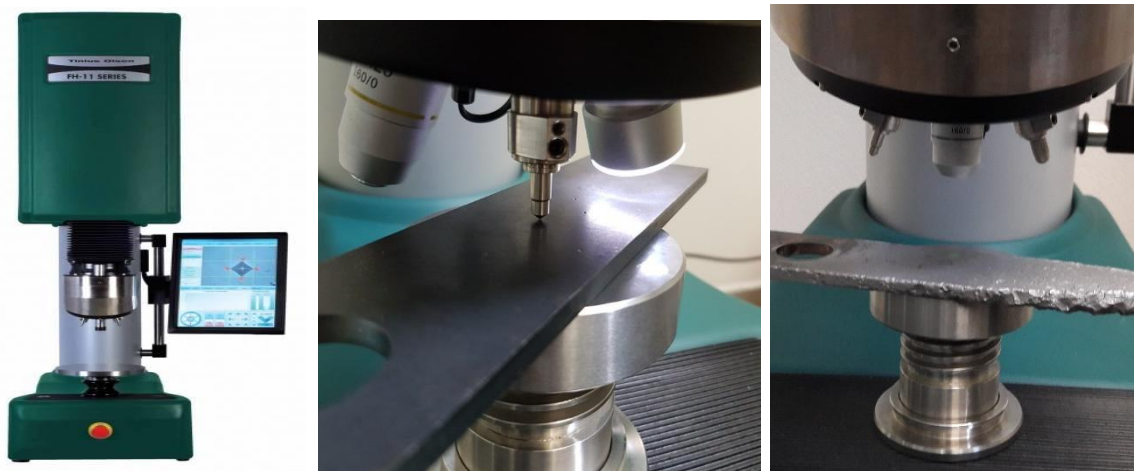
Figure 8: Used FH11 hardness tester (left), measurement of an undamaged tool (middle) and worn tool (right) [10]
