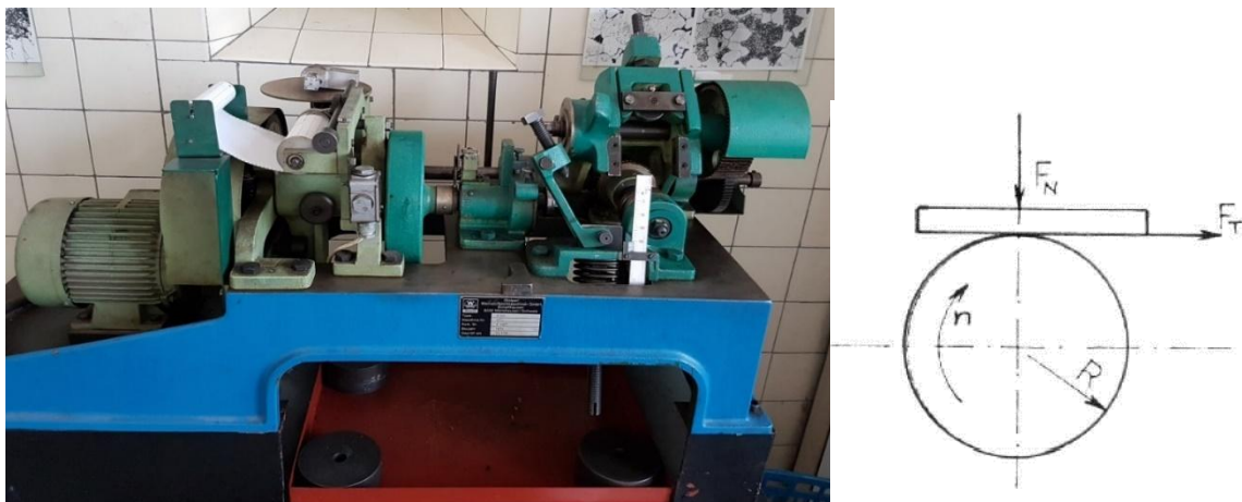
Figure 12: Amsler A 135 testing device (left) and principle diagram of the test (right) [8]
