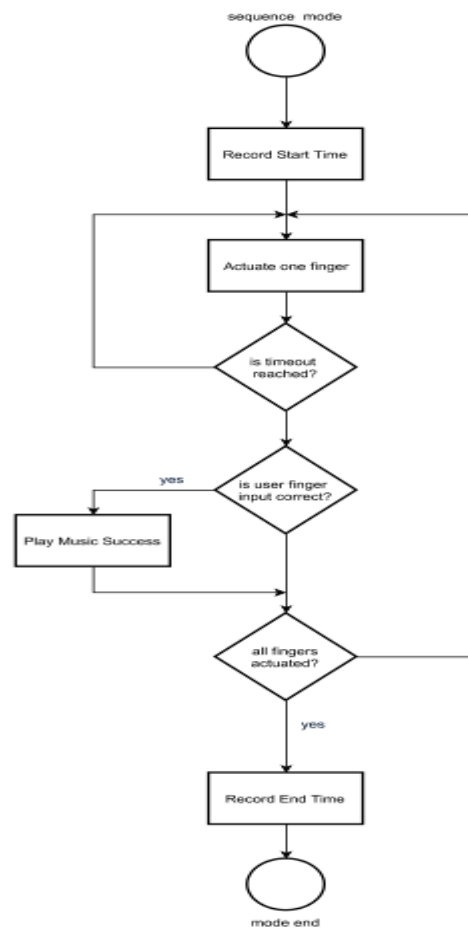
Figure 13:Flow chart for Sequence Mode operation
