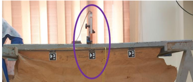
Figure4. Vertical displacement was applied at the mid-span of a sample
