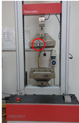
Figure2. Testometric machine (M500/50CT) and the artificial target fixed in the movable jaw
