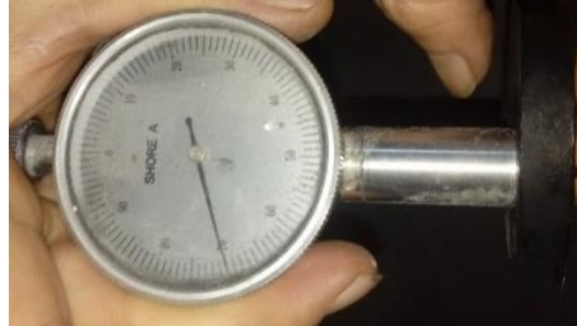
Figure 9: Shore-A hardness testing on rubber sample hardness
