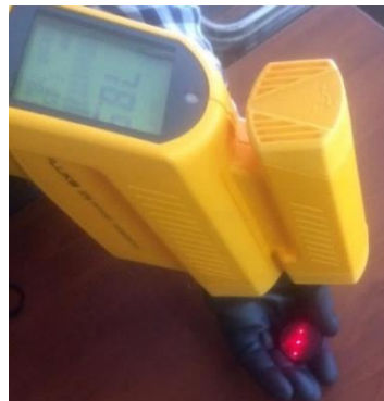
Figure 10: Specimen temperature measurement
