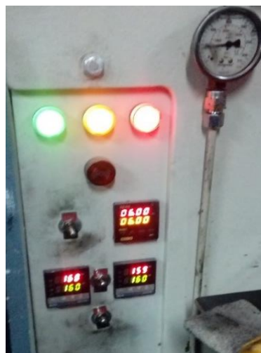
Figure 7: Mold temperature and time control unit
