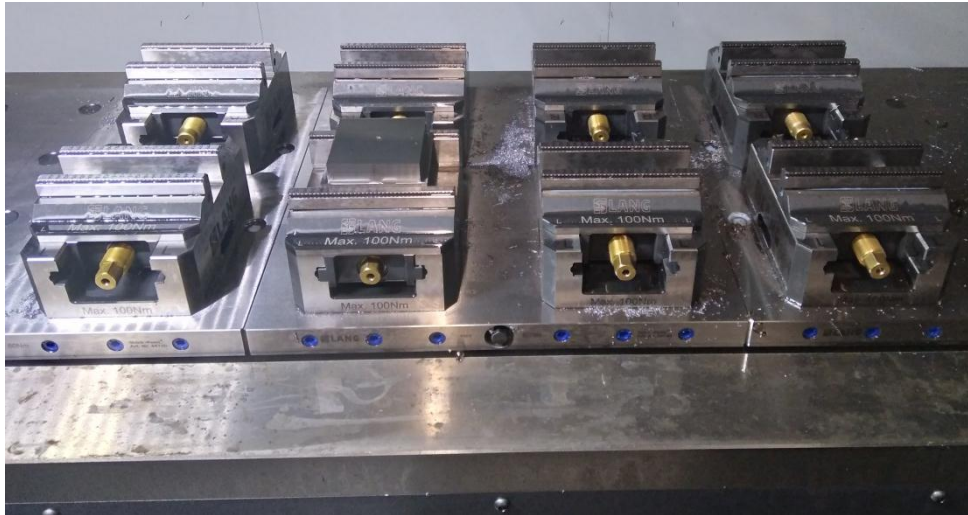
Figure 5: Picture of LANG brand zero-point vice work holdings used at the company.
