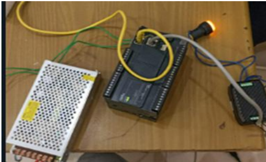
Figure 2:PLC connected with PZEM-017 sensor module
