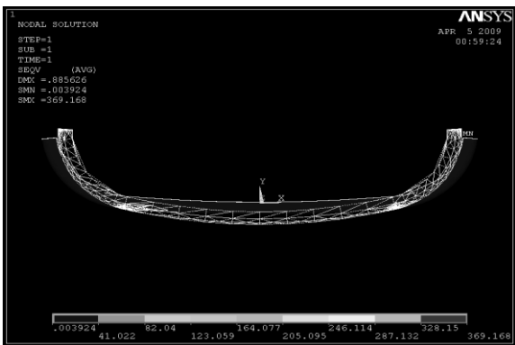
Fig 7.1 Stress Distribution for Steel Bumper
