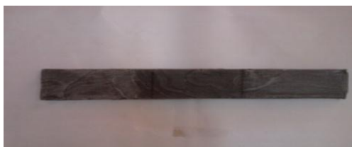
Figure 2.3: Fly ash filled polypropylene composite sample
