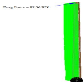
Figure 2.Wind load on windmill tower
