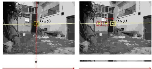
Fig. 4. Correspondence using window – based matching (rectified images)
