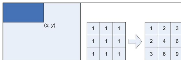
Figure 1. Integral image generation. The shaded region represents the sum of the pixels up to position (x, y) of the image. It shows a 3×3 image and its integral image representation.
