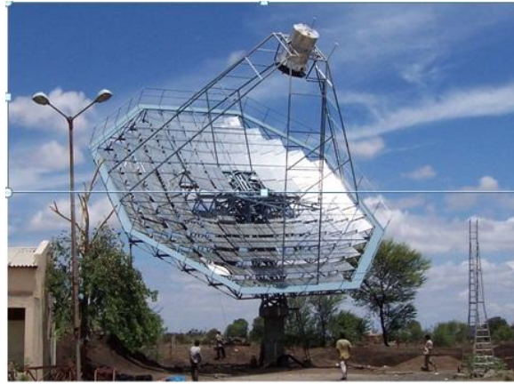
Fig. 3: ARUN solar concentrator system, Clique Consultants
