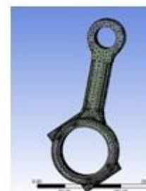
Fig 3. Meshed model of Connecting Rod
