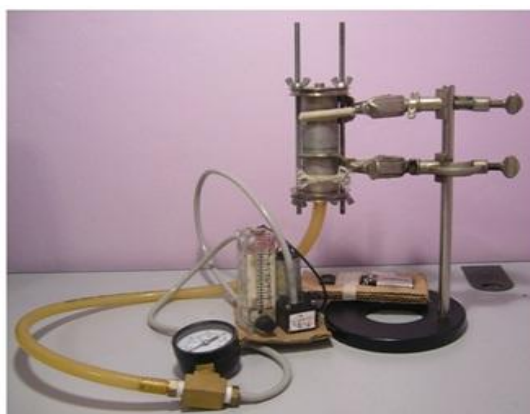
Fig. 1. The two-stage personal cascade impactor.
