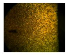
4 % Nital etched sample shows carburizing case depth Upto 0.6 mm at 500X magnification range.
