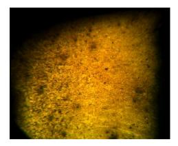
4 % Nital etched sample shows carburizing case depth Upto 0.8 mm at 500X magnification range.
