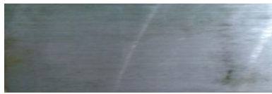
Fig V: Transverse cracks on observed after etching with HCL
