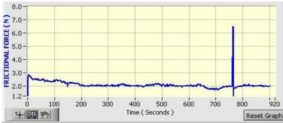
Fig.16. Frictional Force (N) V/s Time (Seconds) at load 20N for 20wt% Al_2O_3
