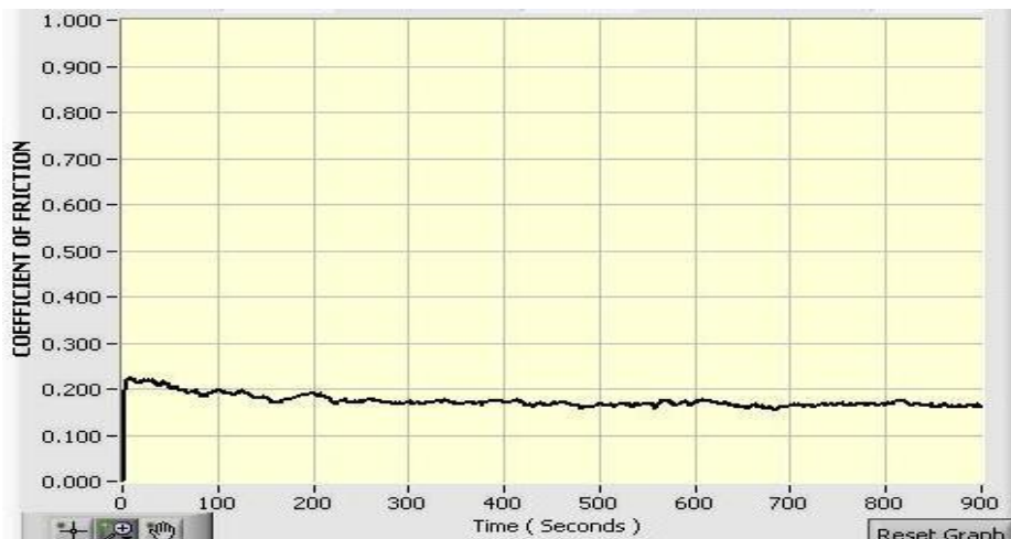
Fig.12. Coefficient of Friction V/s Time (Seconds) at loads 10N for 20wt% Al 2 O 3
