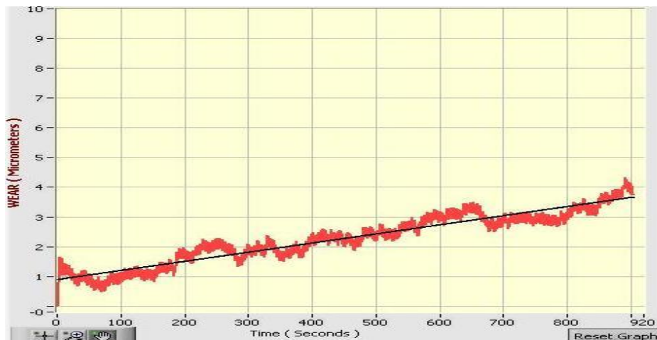
Fig.11. Wear (Micrometers) V/s Time (Seconds) at load 10N for 20wt% Al 2 O 3
