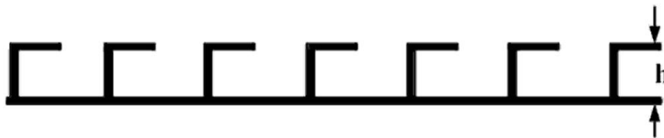
Figure 2. Cavity-loaded corrugations Such corrugations have been applied in horn-antenna design, but they are very expensive to machine. The relative bandwidth is about 2.4 [39].
