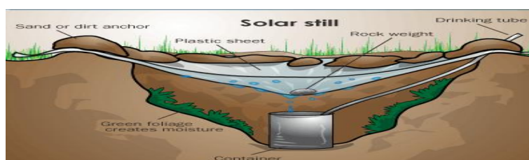
Figure 3: Pit type solar still
