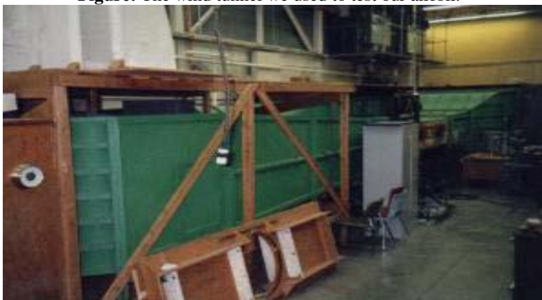
Figure: The wind tunnel we used to test our airfoil.
