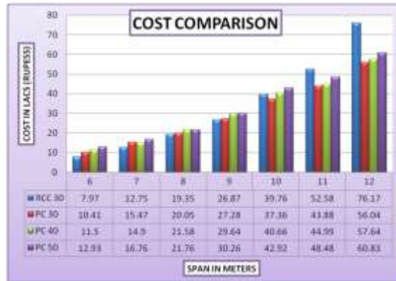
Figure 1: Variation of Cost with Span of Slab
