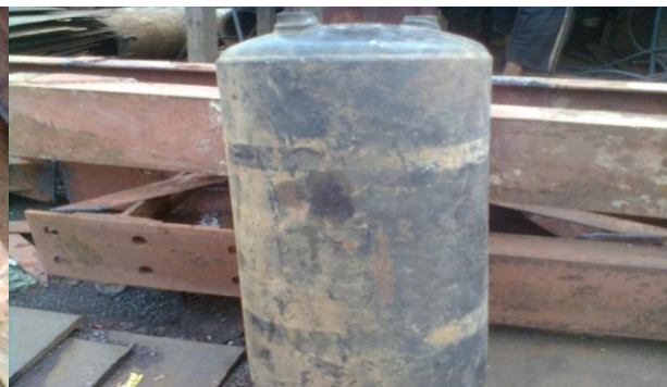
Fig.2.2-Air Tank (Front View)
