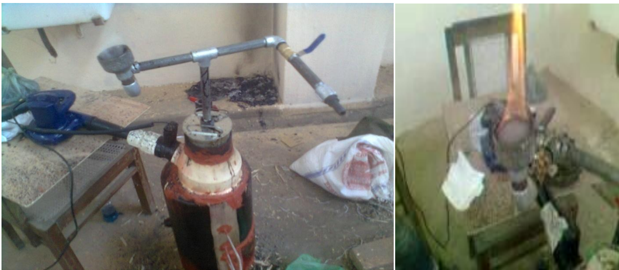
Fig. 3.2- Experimental setup and burning flame in the burner
