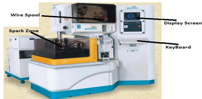
Fig. 2: CNC Wire cut EDM is used for experimentation
