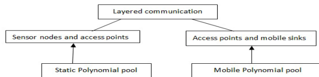
Figure 4.3 Key Pool Segregation
