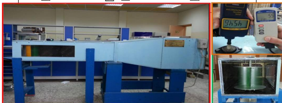
Figure (3): Schematic drawing & the Experimental rig with Savonius blade model.
