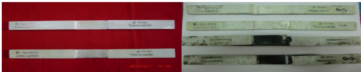
Fig. 2: Tensile test specimens before and after test
