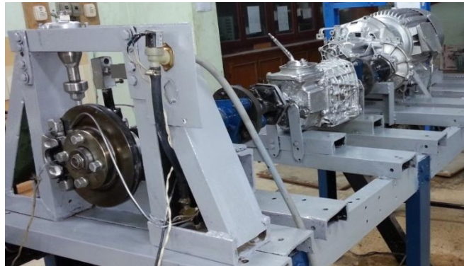
Fig. 1 Main components of the brake dynamometer.
