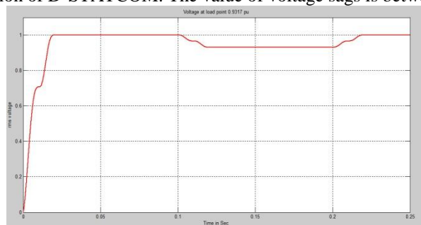
Figure4.2(a).voltage at load point is 0.9317 p.u TLG
