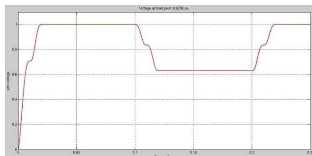
Figure4.1(a).voltage at load point is 0.6296 p.u TLG
