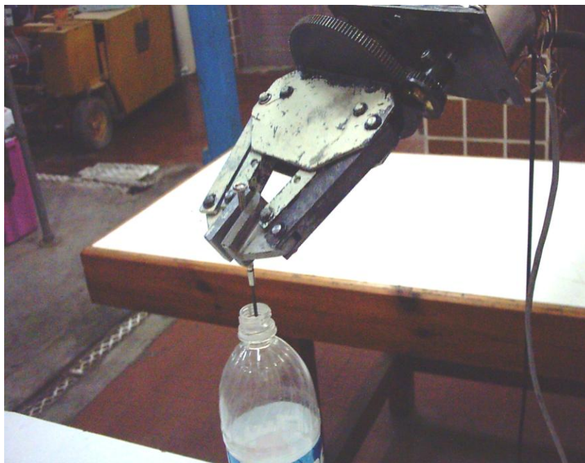
Figure 12 Experiment 2, place the screw driver inside a bottle of small diameter hole
