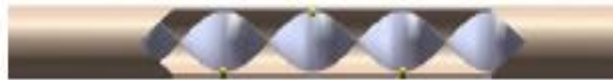
Figure 3. Schematic view of the twisted tape inserted tube separated from the tube inner surface with tefflon rings.
