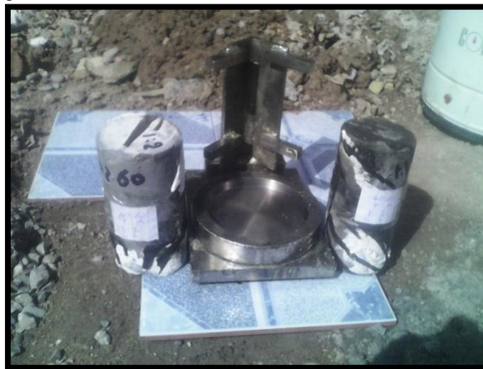
Fig. 2. Capping plate and device.
