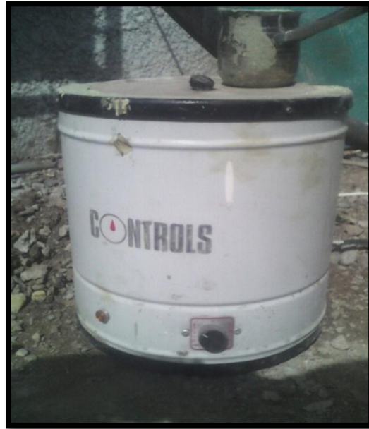
Fig. 3. Capping furnace (Controls Co.) Italy.
