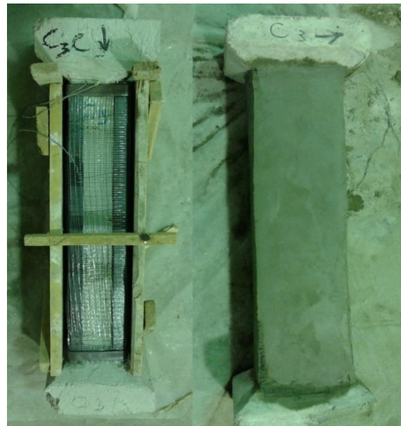
Figure 6 Form shape used for cement mortar
