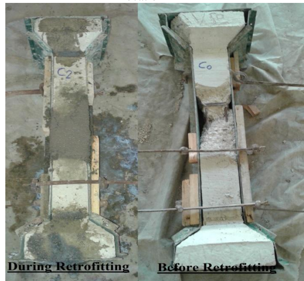
Figure 4 Details of retrofitting columns with Grout mortar.
