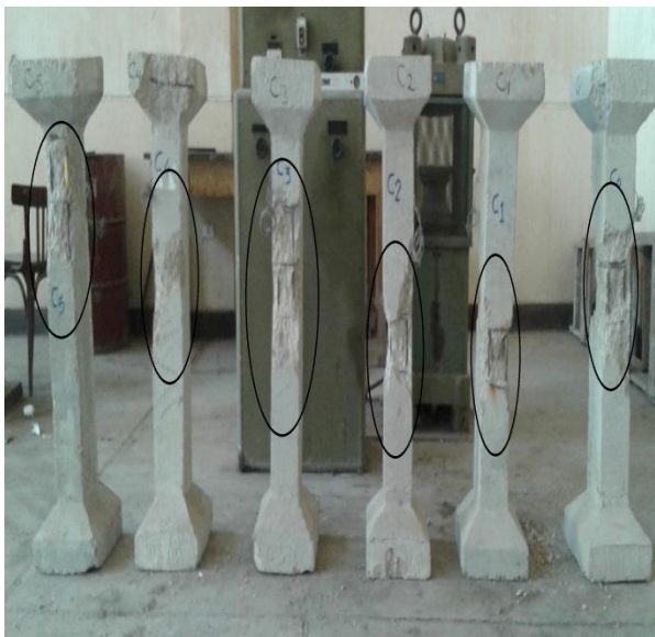
Figure 3 Specimens after testing before retrofitting.
