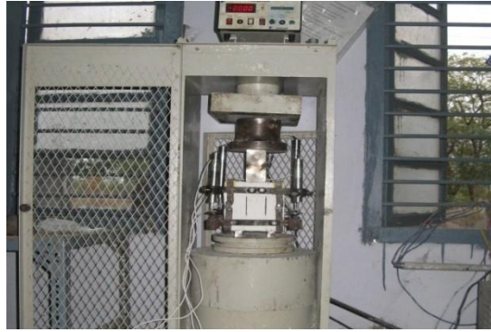
Plate 4. Test setup for DCN specimen
