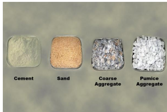
Plate 1. Ingredients of concrete
