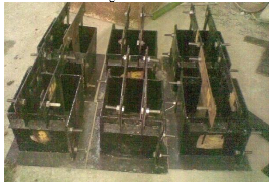
Plate. 2 View of the moulds with double centered notches
