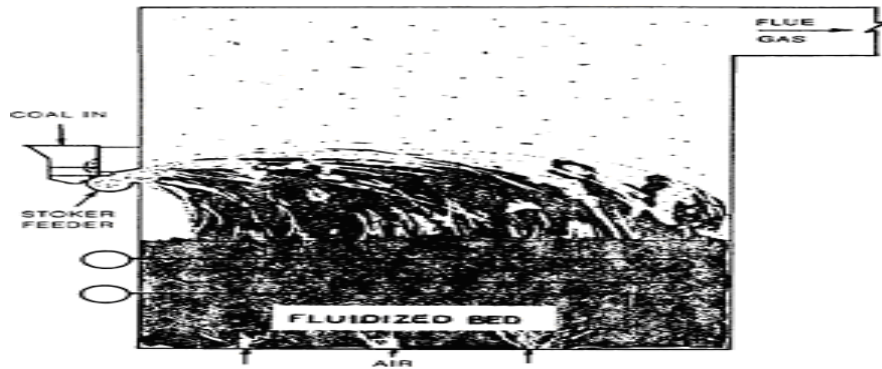
Fig 13: Bubbling Bed Boiler
