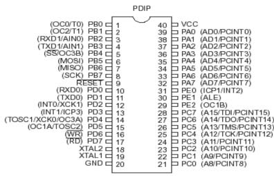
Figure.3 Pin diagram of ATmega162 Microcontroller
