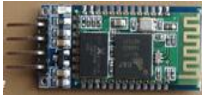
Fig.5 Bluetooth Module: JY-MCU BT_BOARD V1.3
