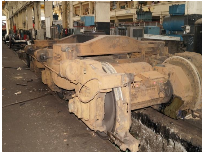
Conventional FLEXICOIL bogie, CO-CO Type of WAP-4 Locomotive.
