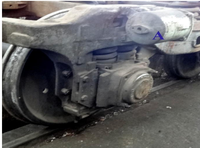
'A' shows brake cylinder.
