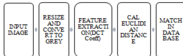
Fig. 5: Block diagram to Calculate Euclidian Distance
