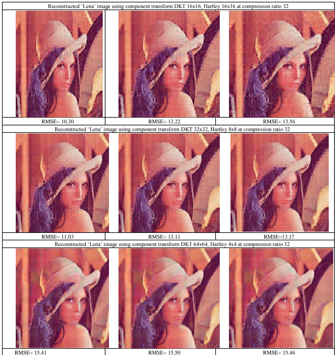
Fig. 17 Reconstructed 'Lena' image using DKT-Hartley hybrid wavelet, multi resolution and hybrid transform with component sizes 8x8 and 32x32 i.e. (8-32), (16-16), (32-8) and (64-4) respectively
