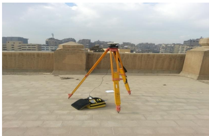
Figure (2) shows the GPS Receiver over the simulated bolts
