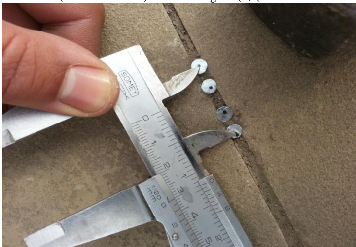
Figure (1) shows the distances between the bolts as well as the vernier scale.
