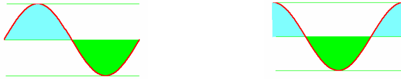
Fig. 1: The area under a sine and a cosine wave over one period is always zero.
