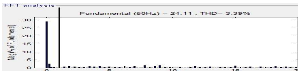
Fig 15: Current harmonics after transformer for Connection B
