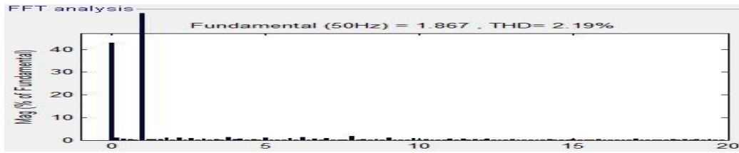
Fig 7: Current harmonics before transformer for Connection A
