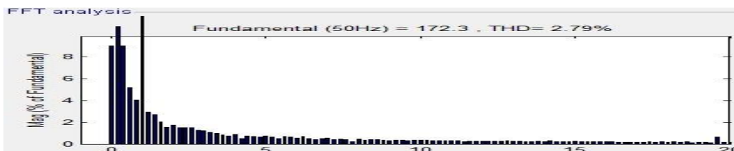
Fig 19: Current harmonics before transformer for Connection C
