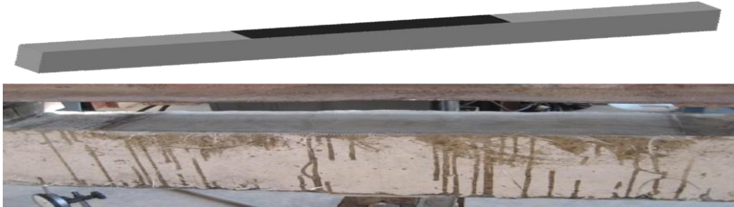
Figure 3.36 Top FRP of Beam TB1 before Testing
