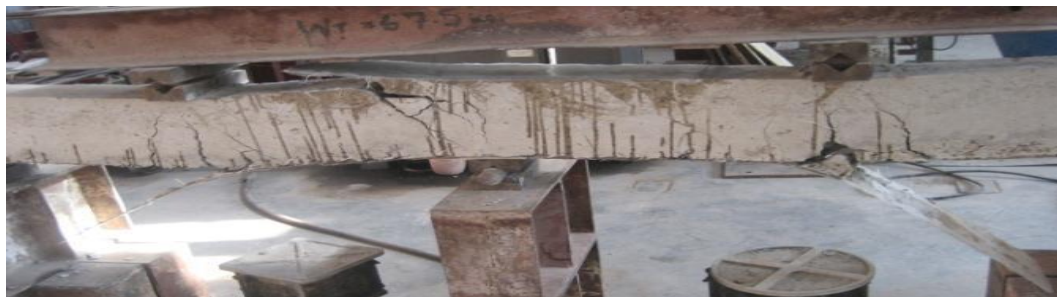
Figure 3.37 FRP sheet separations without concrete
