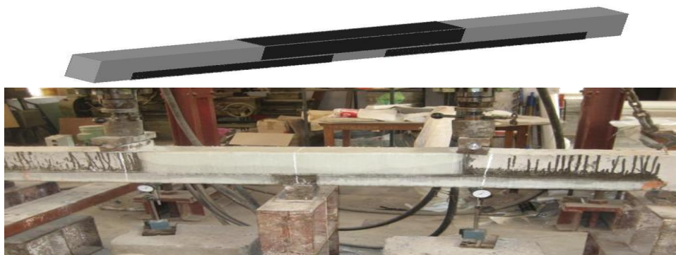
Figure 3.31 Strengthening pattern of SB8
