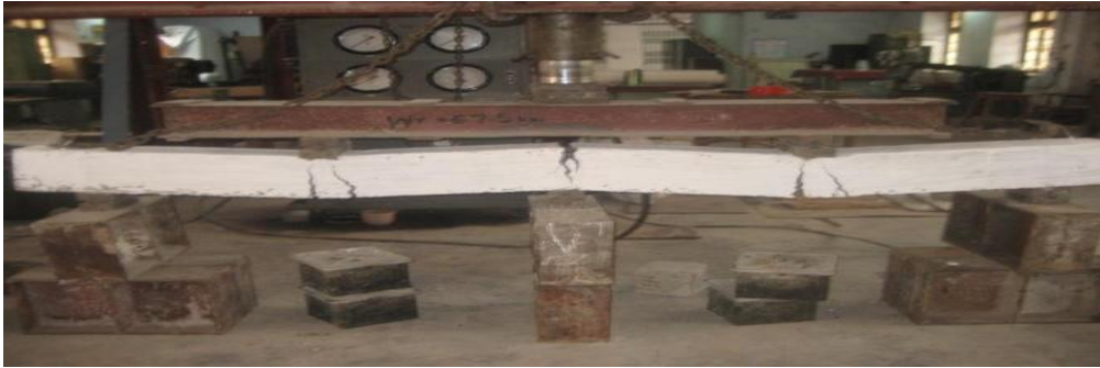
Figure 3.12 Flexural failure of CB1
