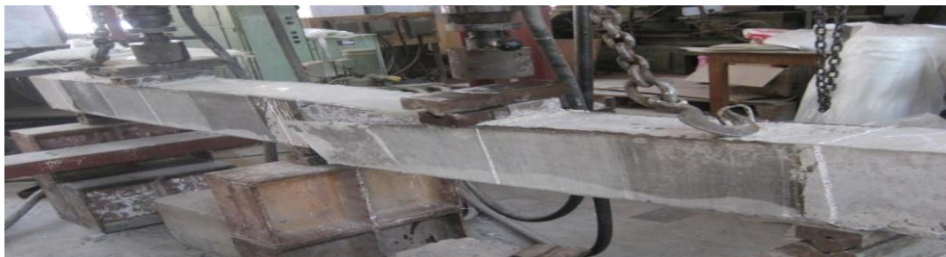
Figure 3.41 Failure of beam TB3
