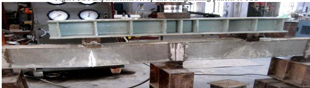
Figure 3.39 Failure of the beam by tensile rupture
