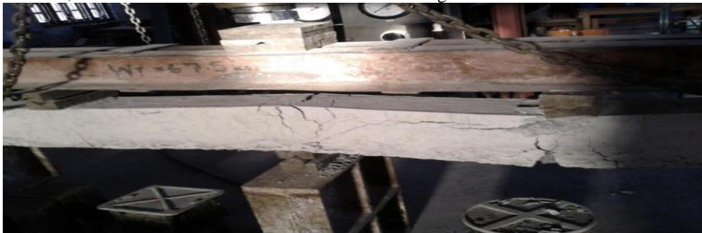
Figure 3.13 Control Beam, CB2 after failure
