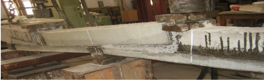
Figure 3.32 Failure of SB8 by debonding of GFRP
