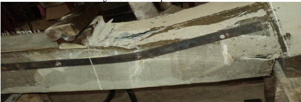
Figure 3.35 Magnified view of Debonding
