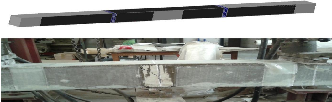
Figure 3.24 Cracking pattern at lower load value
