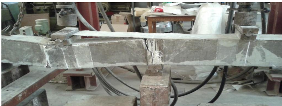
Figure 3.23 Failure of the beam by tensile rupture
