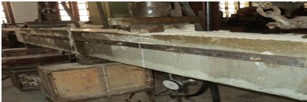
Figure 3.33 Strengthening and anchoring pattern of SB9
