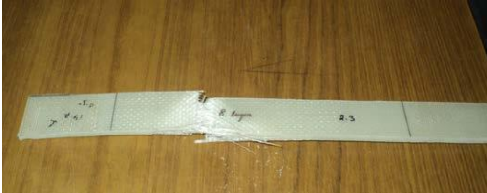
Figure 3.10 Specimen failure after tensile test
