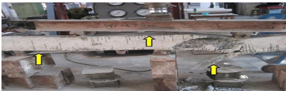
Figure 3.15 Debonding failure of FRP
