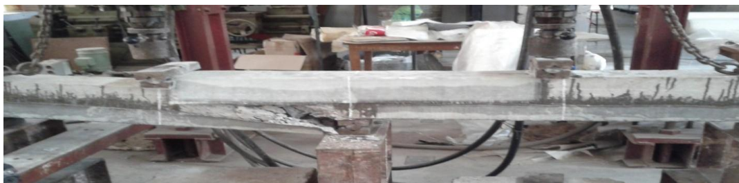
Figure 3.30 Magnified view of shear crack and debonding of GFRP
