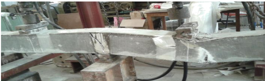
Figure 3.25 Rupture of GFRP sheet at mid section of the right span
