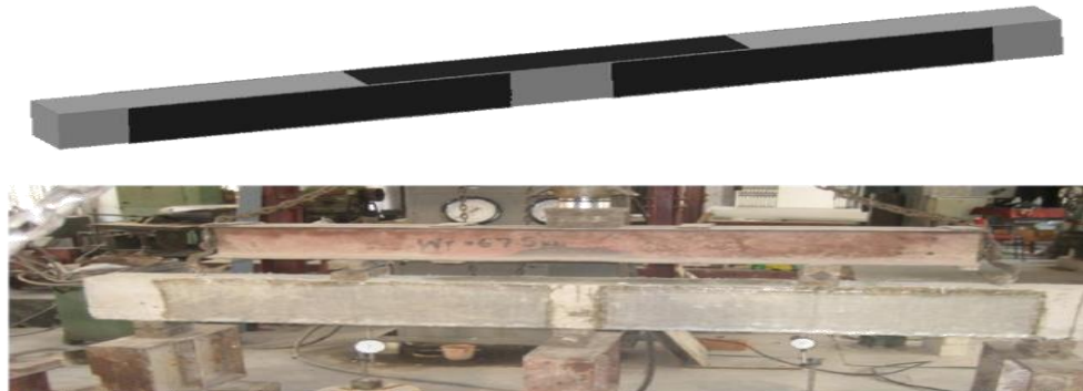
Figure 3.19 U-jacketed GFRP wrapped on the Beam SB3
