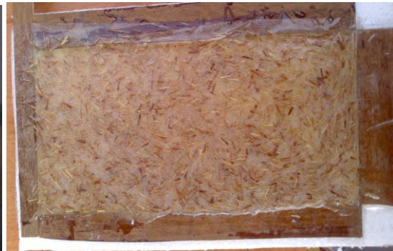
Fig 7: Mould Box with treated fibers and resin mixture
