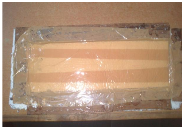
Fig 1: Mould Box fibers and resin mixture
