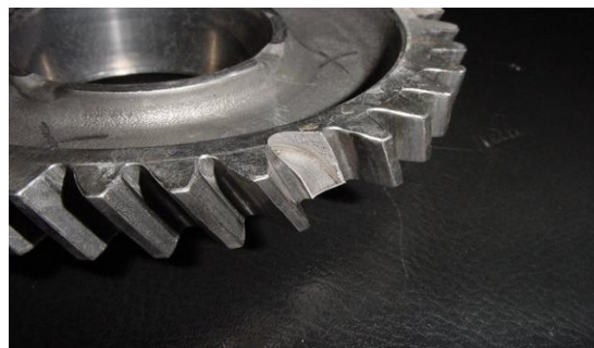
Fig 1. Fatigue failure of gear tooth. (www.google.com)
